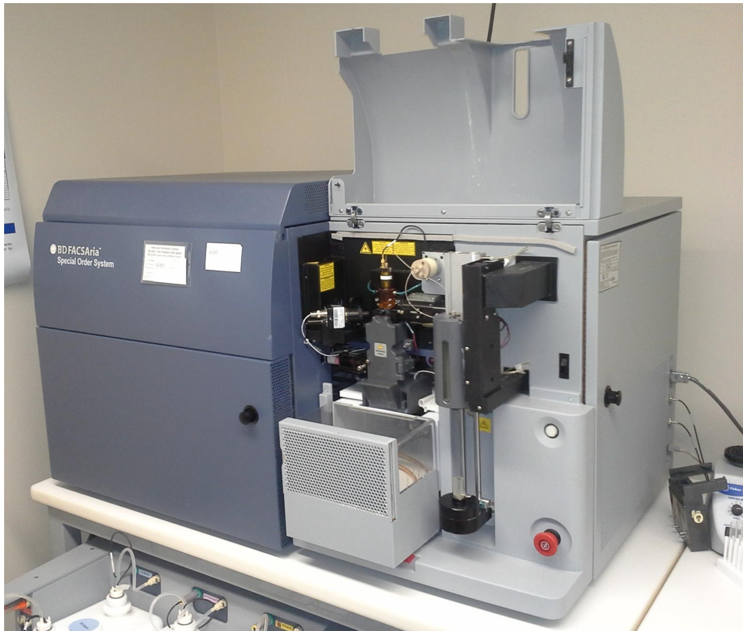
SIXTEEN PARAMETER SYSTEM WITH 2 LIGHT SCATTER AND 14 FLUORESCENCE DETECTORS
